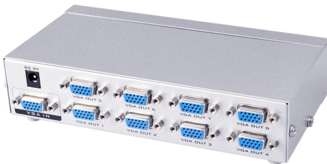
Splitter VGA 8 puertos 150 MHZ Ref: SVG-07
